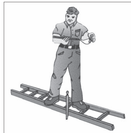
Fig. 3: Proper location for inserting temperature probe
