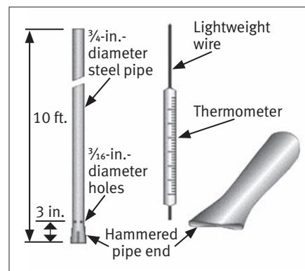
**Fig. 2: Proper procedure for monitoring hay temperatures**
